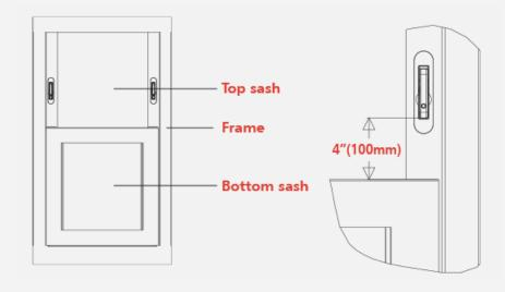
Position opening control device on sash as shown and align the bottom of the restrictor arm on the pencil mark.
