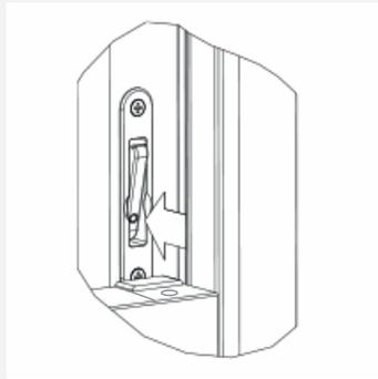
1. Disengage opening control devices on each side
