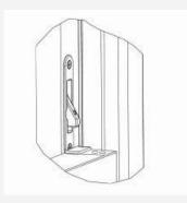
3. Lower bottom sash, opening control device resets
