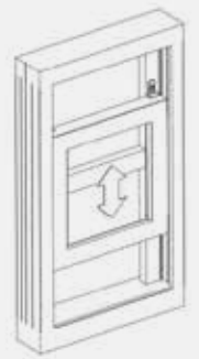
Clear opening cannot exceed 4 inches
