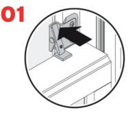
Push top to re-engage window opening control device
