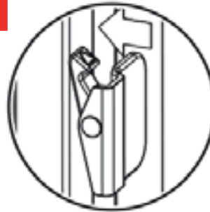
Disengage window opening control device
