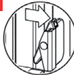
Pull top to re-engage window opening control device
