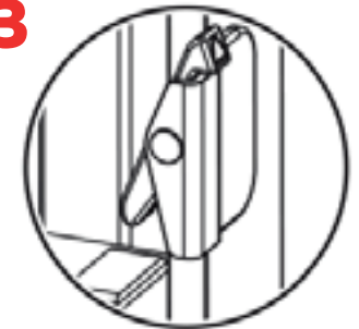
Lower bottom sash. Opening control device resets
