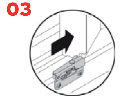
To manually re-engage window opening control device
