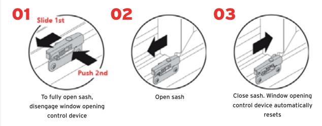
To manually re-engage window opening control device
