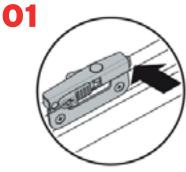
Push end of arm to re-engage window opening control device
