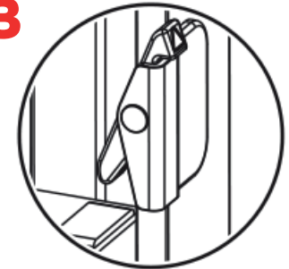
Lower bottom sash. Opening control device resets
