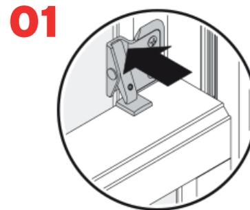
Push top to re-engage window opening control device
